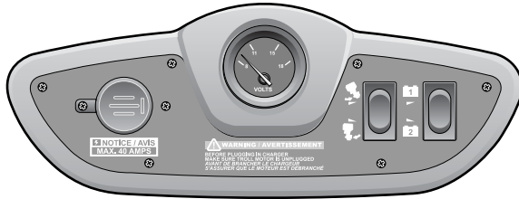
FIGURE 4-4 12 OR 24 VOLT BOW TROLLING PANEL
